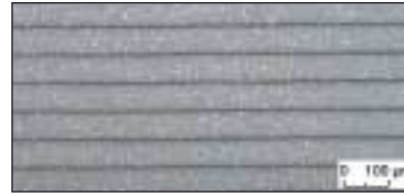
Piezoceramic layers in a monolithic actuator (LVPZT).
