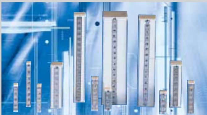
Fig. 39 a. PICMA® actuators are made with ceramic-only insulation and can dispense with any polymer coating. Result No measurable outgassing, insensitive to atmospheric humidity and a wider operating temperature range.
