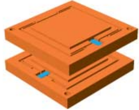
Fig. 50 a. Working principle of a stacked XY piezo stage (serial kinematics). Advantages: Modular, simple design. Disadvantages compared with parallel kinematics: More inertia, higher center of gravity, moving cables (can cause friction and hysteresis). Integrated parallel metrology and active trajectory control (automatic off-axis error correction) are not possible.
