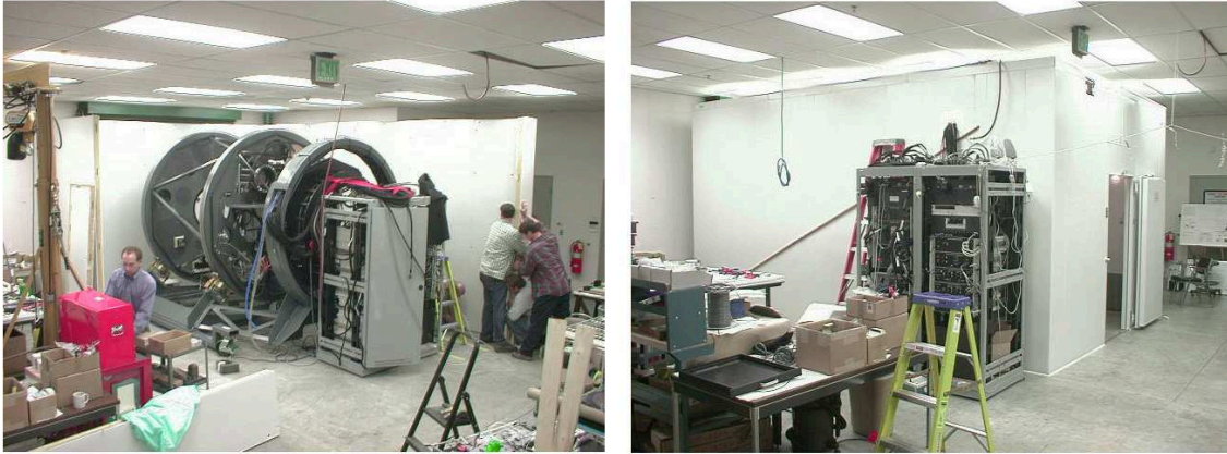
Fig. 36. A commercial freezer enclosure was erected around IMACS for thermal testing in the lab in Pasadena. The Bally freezer came with a refrigeration unit with dehumidifier; an independent dehumidifier was added to keep humidity low during warm up.
