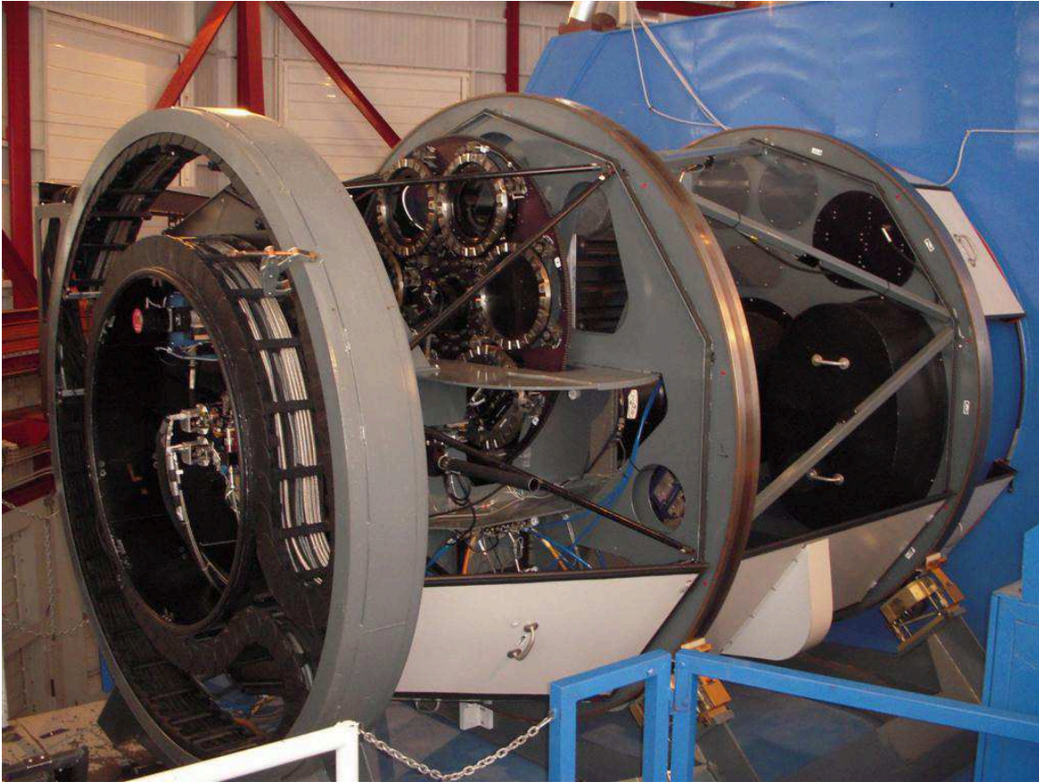
Fig. 20. IMACS installed at the west Nasmyth platform of Baade, with most of the enclosure panels removed. This photo shows the carriage with its self-steering rollers supporting the rotation IMACS structure assembly. The rotating assembly consists of three sections. (1) Main structure — Two monocoque disks ('Forward' and 'Main' Optical Support Structure, FOSS & MOSS) connected by the grey-square-tube main truss. This section encloses the collimator and its baffle, and the f/4 train: Filter Server, Shutter, f/4 Camera, and Mosaic1 CCD camera (all far side, not visible). (2) Forward compartment, the short projection from the FOSS disk to the Nasmyth instrument rotator. This section encloses the field lens, the Mask Server, the three guiders, and the calibration unit. (3) Aft compartment — The secondary truss (black bars) supports the cantilevered, rotating portion of the utility wrap at the back of the instrument. In this section is the MOSS Box, the weldment to which collimator, f/2, and f/4 cameras are attached — in other words, the spectrograph). Also visible is the primary structure (wheel) of the Disperser Server; the gratings and grisms face forward and are identifiable by the index rings used to latch a selected unit to the spectrograph. Also enclosed in the aft compartment are The f/2 train: Filter Server, Shutter, f/2 Camera, Detector. The Filter Server and Detector are slightly visible within the utility wrap.
