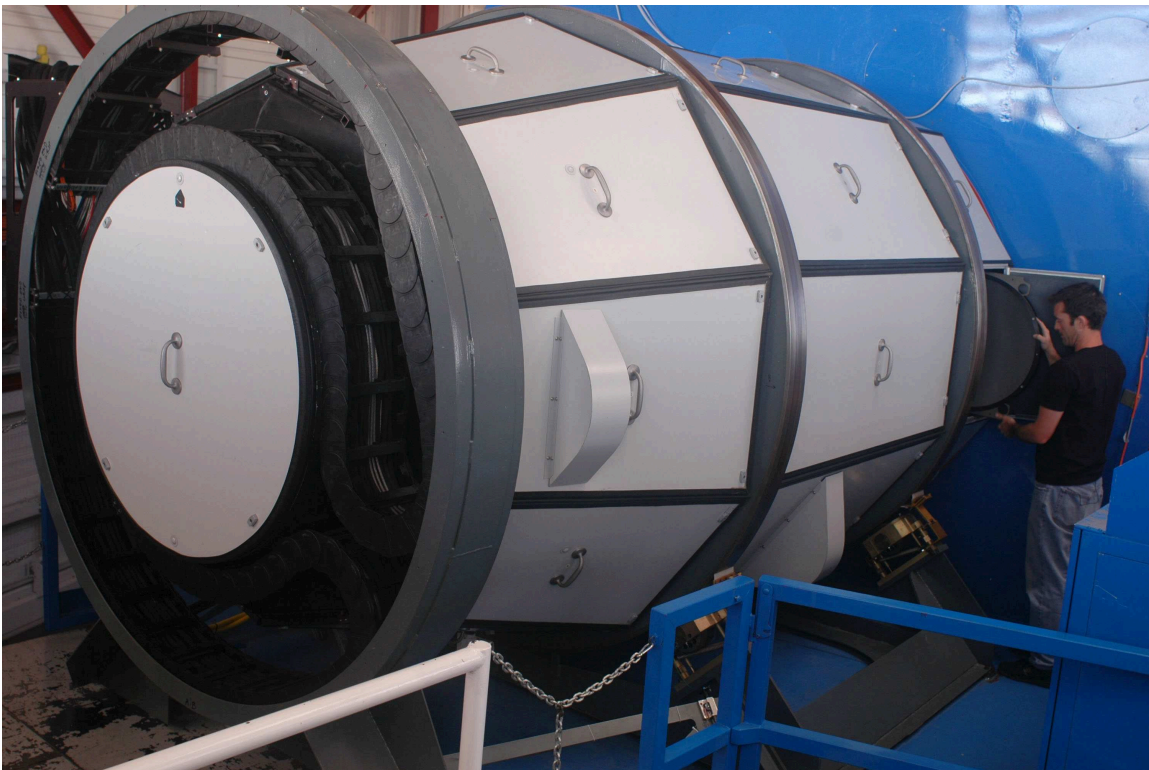
Fig. 1. IMACS on the west Nasmyth platform of the Magellan-Baade telescope. Tyson Hare installs a multislit mask into the Mask Server (at the telescope focal surface). The spectrograph structure is covered by insulated aluminum panels with butted vinyl seals. The cable wrap is the black structure seen at the back.
