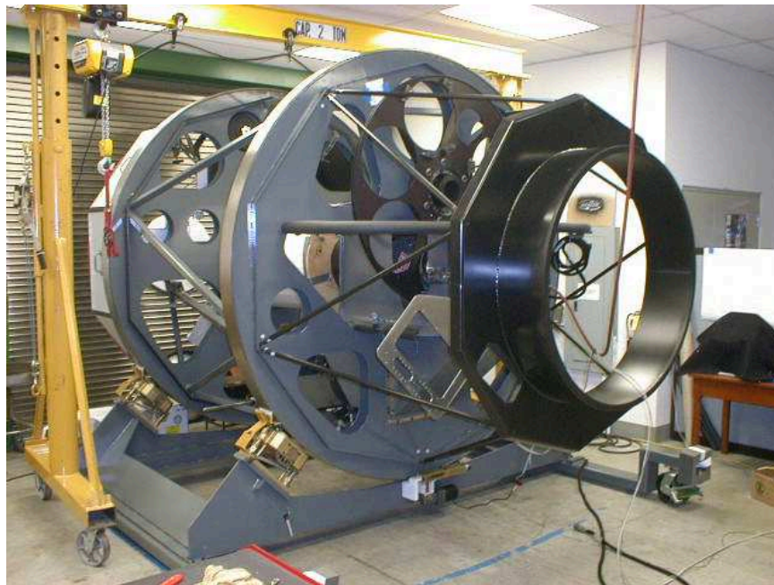
Fig. 21. An early stage of assembly of IMACS in the Carnegie Observatories shops. This photo shows the carriage, with its self-steering rollers supporting the rotating part of the IMACS structure assembly. The rotating assembly consists of two monocoque disks connected by the main truss, the secondary truss (black) supporting the cantilevered, rotating portion of the utility wrap, and the Main Optics Support Structure (MOSS). Also visible in the photo is the primary structure (wheel) of the disperser server that carries the spectrograph dispersers and accessories.
