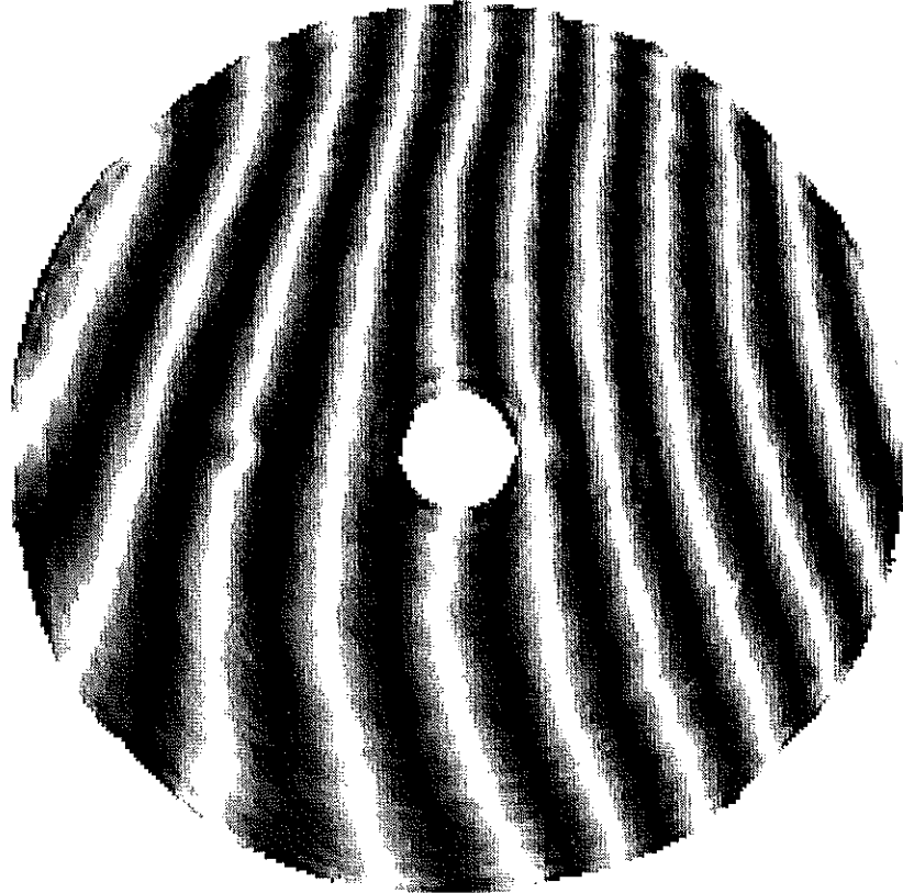
Figure 4. Gray-scale map of the mirror surface and synthetic interference pattern for the original map including astigmatism and spherical aberration. The gray scale covers \pm 350 nm of surface. The displays show the full measured wavefront and include some spurious pixels outside the polished surface.
