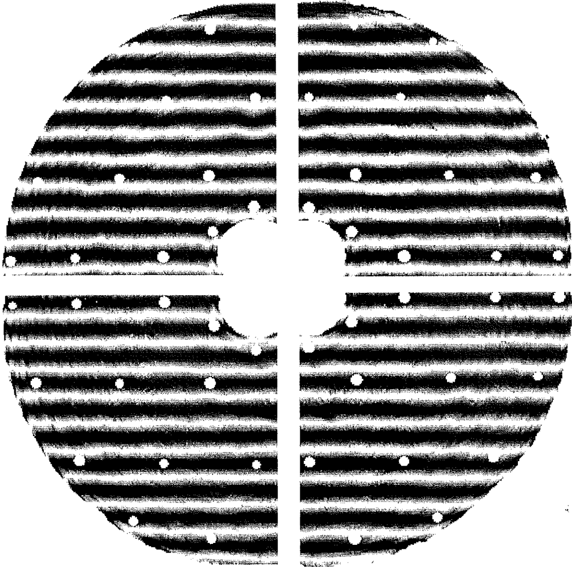
Figure 11. Synthetic interference patterns, calculated at 633 nm, for the 4 subapertures.
