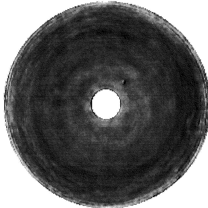
Figure 2. Gray-scale map of the mirror surface and synthetic interference pattern with astigmatism subtracted. The gray scale covers \pm 100 nm of surface.
