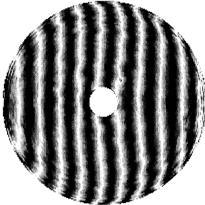
Figure 2. Gray-scale map of the mirror surface and synthetic interference pattern with astigmatism subtracted. The gray scale covers \pm 100 nm of surface.
