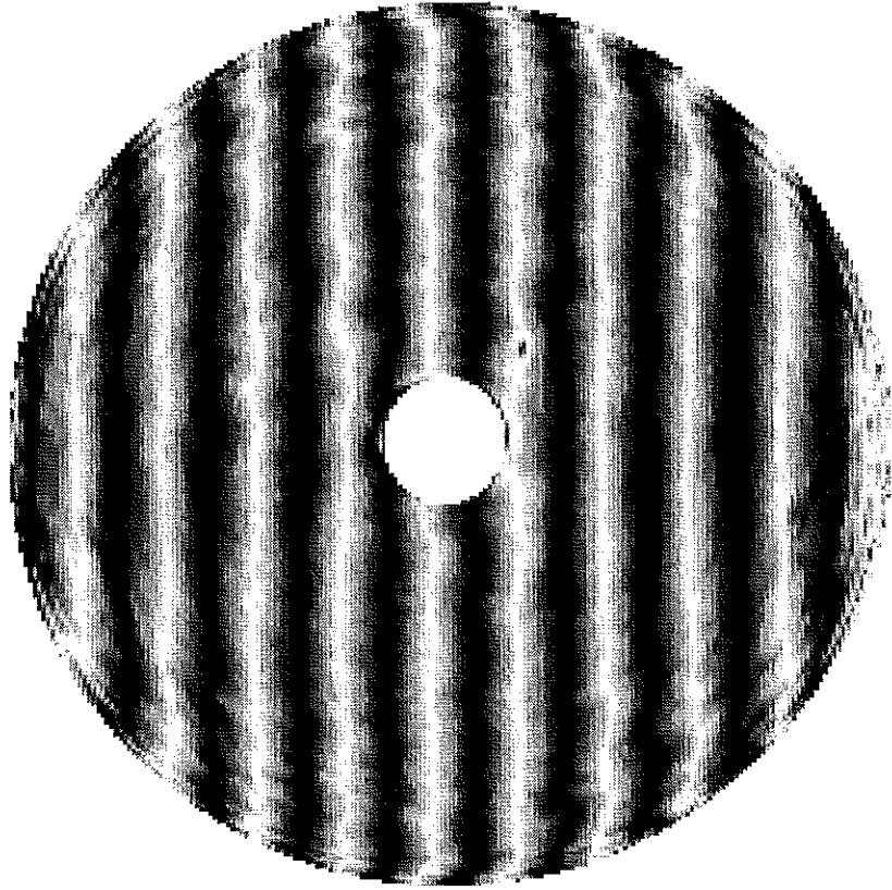
Figure 3. Gray-scale map of the mirror surface and synthetic interference pattern with astigmatism and spherical aberration subtracted. The gray scale covers \pm 100 nm of surface.
