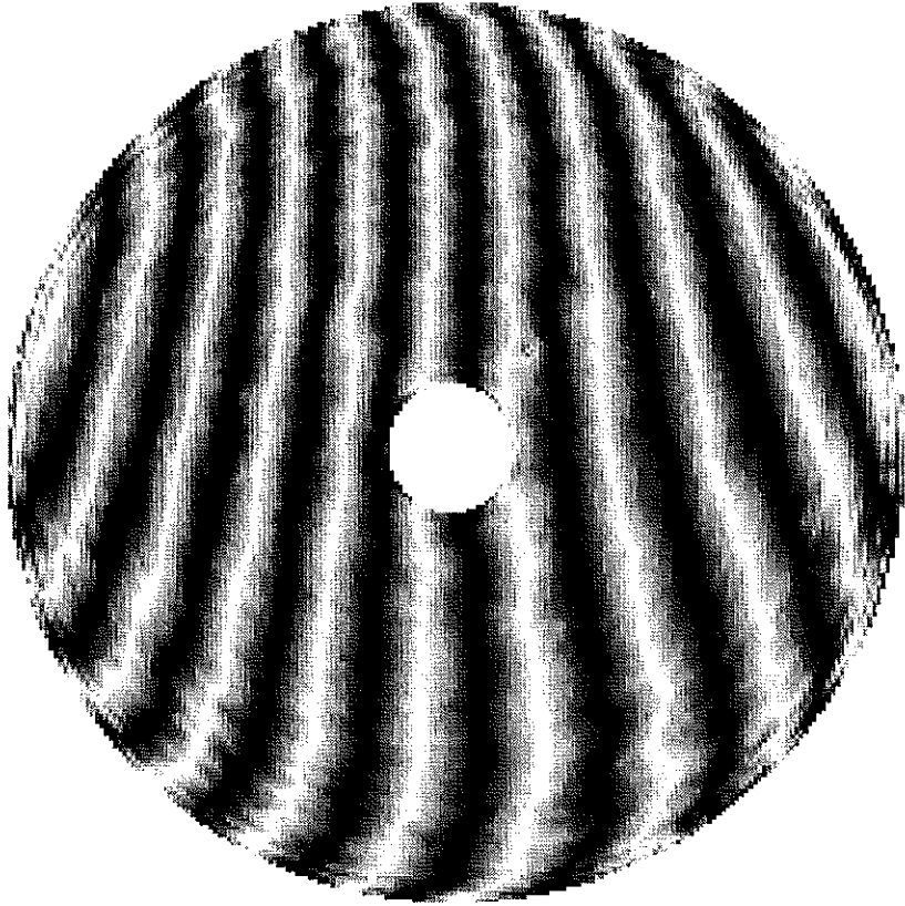
Figure 1. Gray-scale map of the mirror surface and synthetic interference pattern for the original map. The gray scale covers \pm 300 nm of surface.
