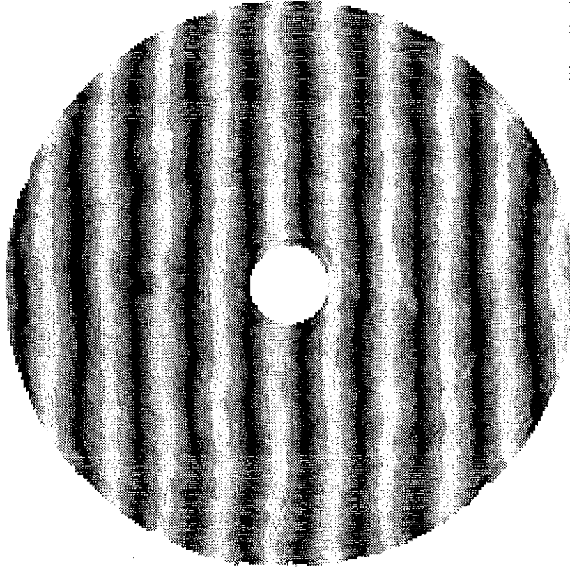
Figure 3. Gray-scale surface map and synthetic interference pattern for the optimized support forces, with astigmatism subtracted. The gray scale covers \pm 100 nm of surface. The rms surface error is 14 nm.
