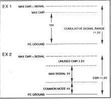
Most manufactures of A/D boards specify the CMR directly from the component data sheet, ignoring the effect of the board level system on that specification. A data sheet of that type might claim 10 volts of CMR. Although this is a factual specification and the designer of the board (or other EE) would be able to translate that into a systems specification, most A/D board owners are confused or mislead by such specs.
