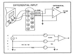
A single ended input has no common mode range because there is only one LOW wire, which is assumed to be at the same level at the signal and at the A/D board.
