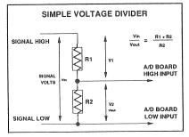
The phenomena of dropping the voltage proportionally is often called attenuation. The formula for attenuation is:
