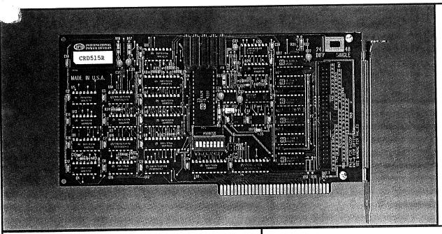
FULL 12 BIT RESOLUTION IN BOTH VOLTAGE and CURRENT RANGES
